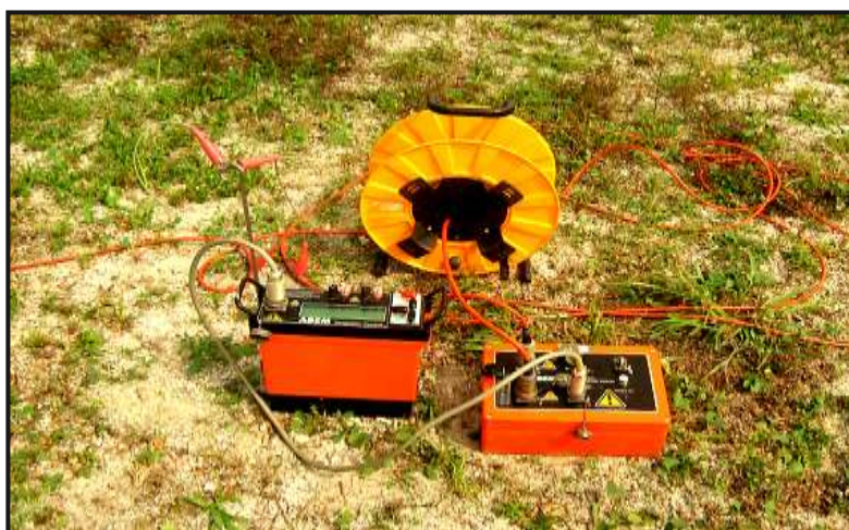
Figure 8: viewing the instrument type SAS1000 applied in geophysical survey
